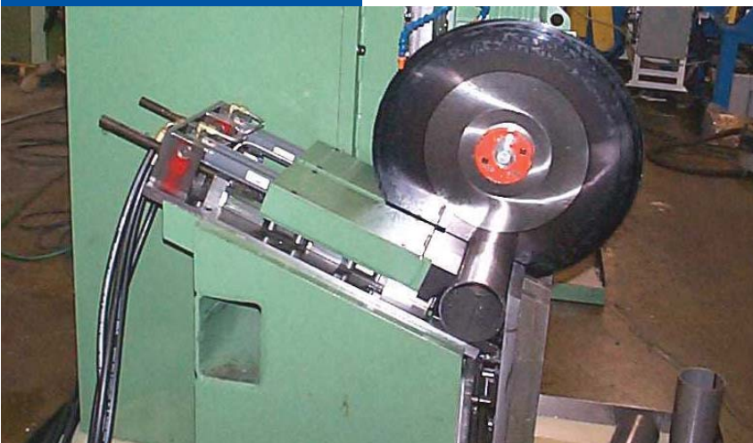
New NAC 20" saw cutting through a large tube
